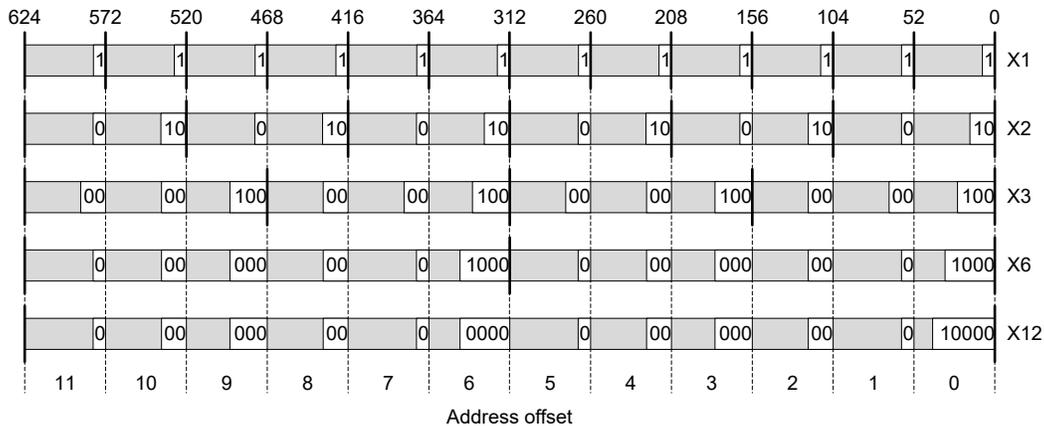
In total, X1 entries require 1 type-group bit per entry, X2 entries require 3 type-group bits per entry, X3 entries require 7 type-group bits per entry, X6 entries require 13 type-group bits per entry, and X12 entries require 27 type-group bits per entry.
