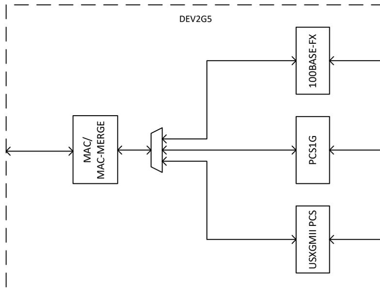
Each of the DEV5G, DEV10G, and DEV25G Port modules have an associated DEV2G5 port module as a shadow device to handle speeds less than or equal to 2.5G.
