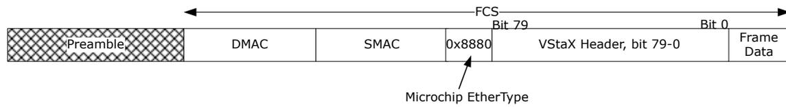
The layout of the 10-byte VStaX header is shown in the following figure. In VStaX context, each switch in a stack is termed a unit.
