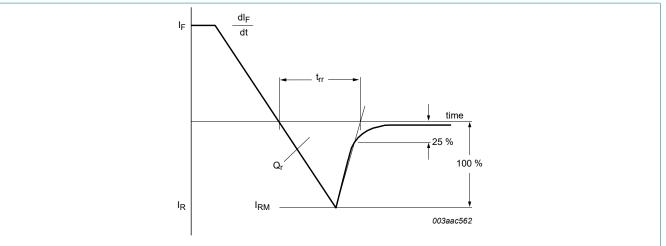
Fig. 12. Reverse recovery definition; ramp recovery
