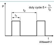
Fig. 13. Duty cycle definition
