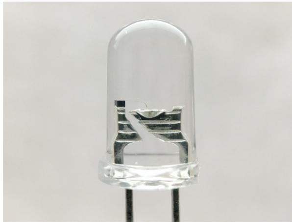
*LED with Built-In Resistor Close Up*
