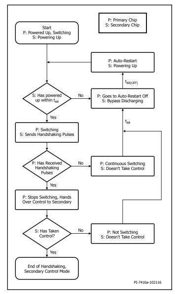
Figure 7. Primary-Secondary Handshake Flowchart.
