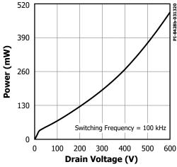
Figure 22. Drain Capacitance Power (INN3977CQ).
