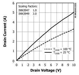
Figure 33. Output Characteristics.
