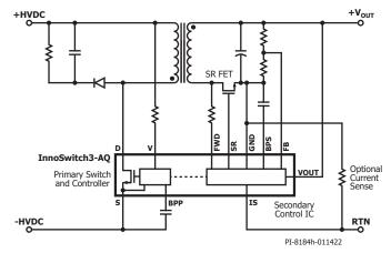
Figure 1. Typical Application Schematic.
