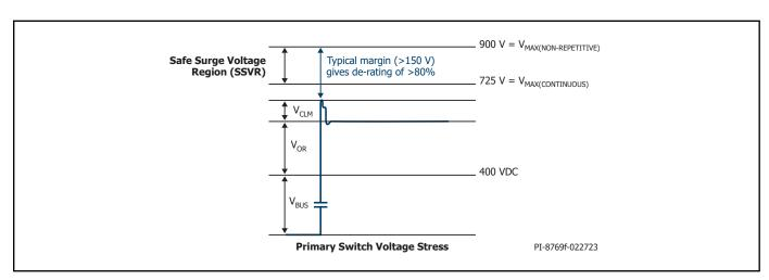
Figure 18. Peak Drain Voltage for 264 VAC Input Voltage.
