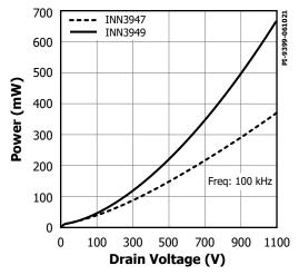
Figure 31. Drain Capacitance Power.
