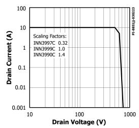
Figure 39. Maximum Allowable Drain Current vs. Drain Voltage.
