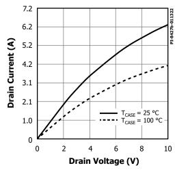
Figure 20. Output Characteristics (INN3977CQ).
