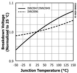
Figure 30. Breakdown Voltage vs. Temperature.
