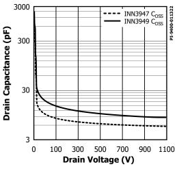
Figure 32.  $C_{\rm OSS}$  vs. Drain Voltage.
