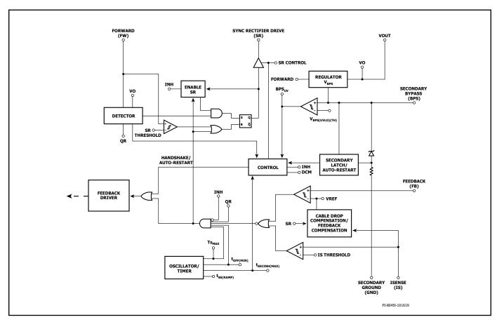
Figure 4. Secondary Controller Block Diagram.
