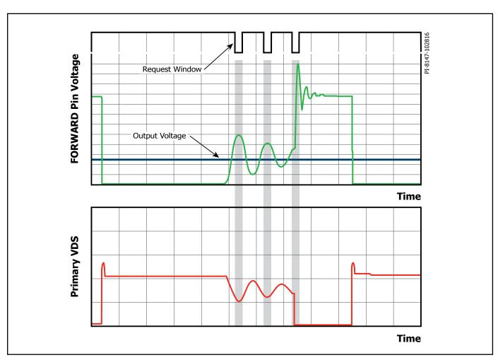
Figure 8. Intelligent Quasi-Resonant Mode Switching.
