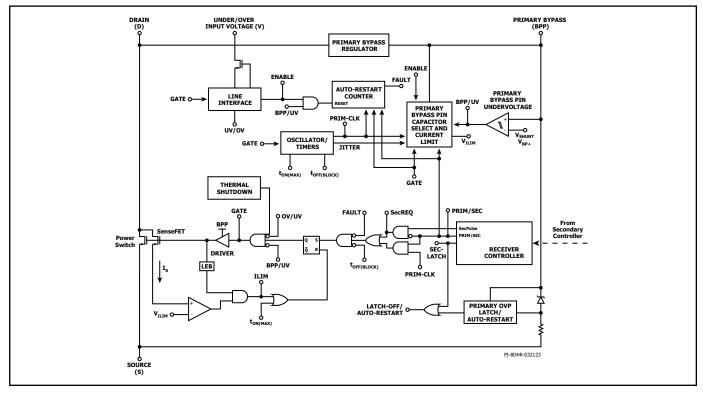
Figure 3. Primary Controller Block Diagram.
