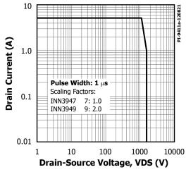
Figure 34. Maximum Allowable Drain Current vs. Drain Voltage.
