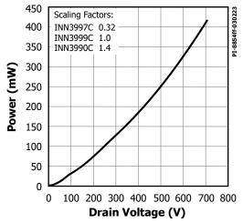
Figure 36. Drain Capacitance Power.
