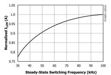
Figure 6. Normalized Primary Current vs. Frequency.
