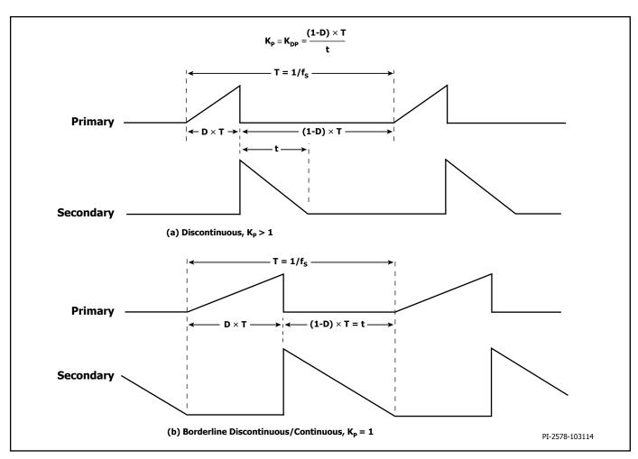
Figure 17. Discontinuous Conduction Mode Current Waveform,  $K_p > 1$ .
