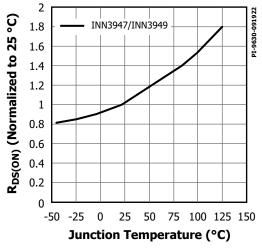
Figure 35.  $R_{DS(ON)}$  vs. Temperature (INN3947/INN3949).
