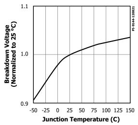
Figure 25. Breakdown Voltage vs. Temperature (INN3977CQ).
