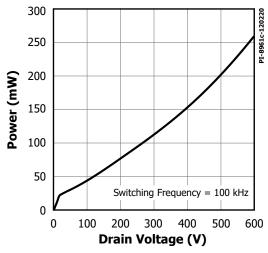
Figure 29. Drain Capacitance Power (INN3996CQ).
