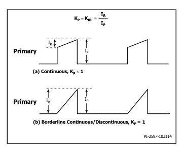
Figure 16. Continuous Conduction Mode Current Waveform,  $K_D < 1$ .
