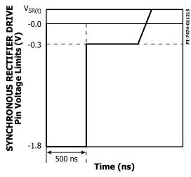
Figure 24. SYNCHRONOUS RECTIFIER DRIVE Pin Negative Voltage.
