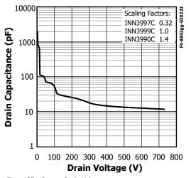
Figure 37.  $C_{OSS}$  vs. Drain Voltage.
