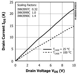
Figure 38. Output Characteristics.
