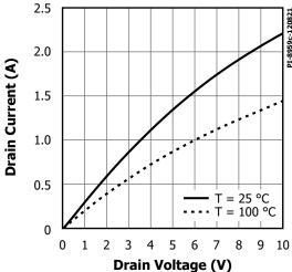
Figure 27. Output Characteristics (INN3996CQ).
