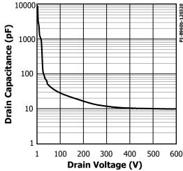
Figure 28.  $C_{\rm oss}$  vs. Drain Voltage (INN3996CQ).
