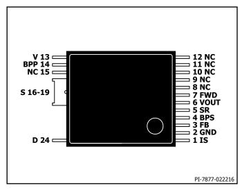
Figure 5. Pin Configuration.
