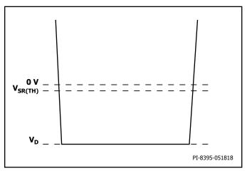
Figure 13. Acceptable FORWARD Pin Waveform before Handshake with Body Diode Conduction During Flyback Cycle.
