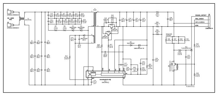
Figure 9. 12 V, 30 W Power Supply.
