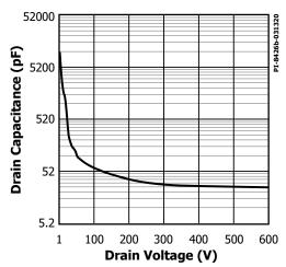
Figure 21.  $C_{oss}$  vs. Drain Voltage (INN3977CQ).
