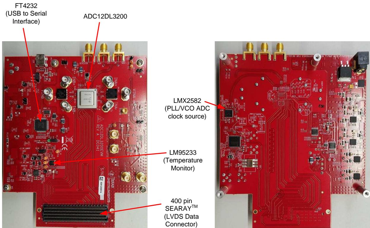
The ADC12DL3200 evaluation module (EVM) is used to evaluate the ADC12DL3200 analog-to-digital converter (ADC) from Texas Instruments. Throughout this document, the terms evaluation board, evaluation module, and EVM are synonymous with the ADC12DL3200EVM.
