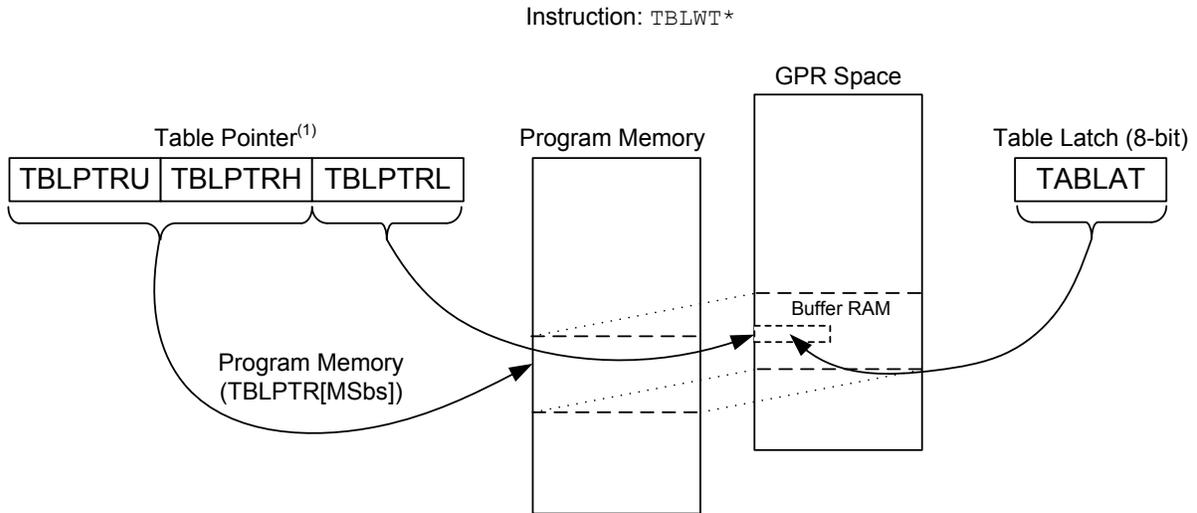
**Note 1:** During table writes the Table Pointer does not point directly to program memory. TBLPTRL actually points to an address within the buffer registers. TBLPTRU:TBLPTRH points to program memory where the entire buffer space will eventually be written with the NVM commands.
