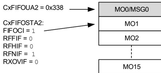
Figure 38-26 illustrates the status of FIFO 2 after MSG0 is read. The user application reads the message from RAM and sets the UINC bit (CxFIFOCON2[8]). The user address increments and points to MO1. The FIFO index is unchanged. The FIFO is empty again. All flags are cleared.
