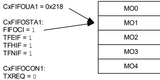
Figure 38-21 illustrates the status of FIFO 1 after three more messages are loaded: MSG1-MSG3. The user address now points to MO4. TFHIF is cleared because the FIFO is now less than half empty.
