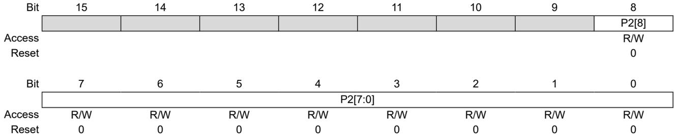
**Bit 8 – P2[8]** Parameter 2 Most Significant bit
