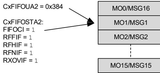
Figure 38-31 illustrates the status of FIFO 2 after the application cleared RXOVIF and read two more messages. RFFIF is clear because the FIFO is not full anymore. The user address points to MO3. The FIFO index has not changed.
