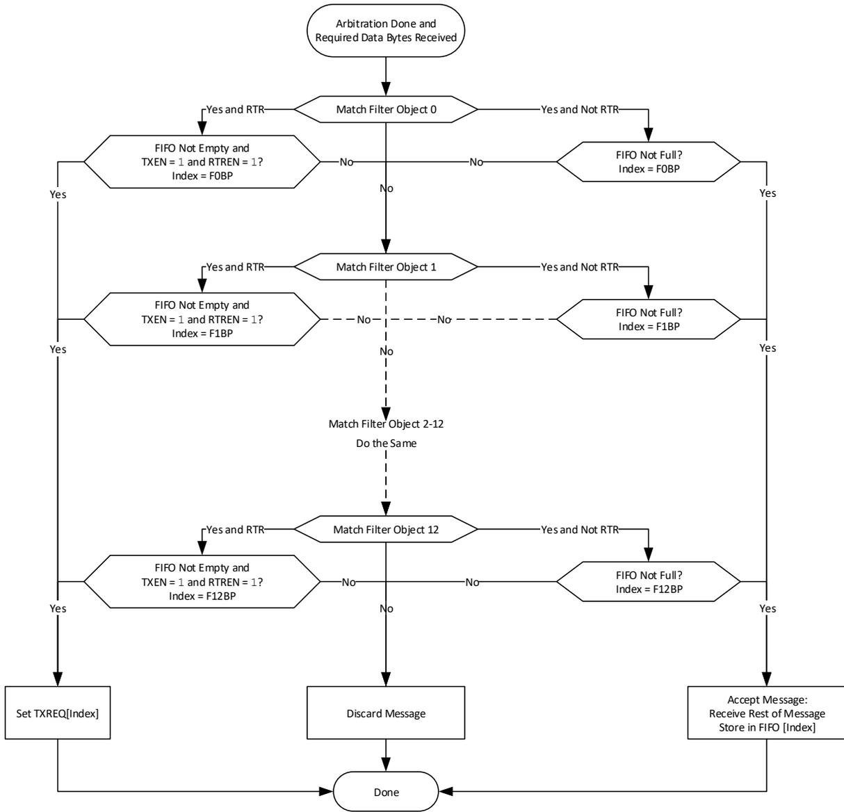
**38.7.2.1 Filtering Standard or Extended Frames**
