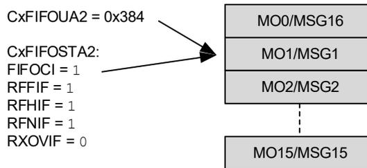
Figure 38-30 illustrates the status of FIFO 2 after one more message is received. Since FIFO 2 is already full, an overflow occurs. The message is discarded and RXOVIF is set. The user address and FIFO index has not changed.
