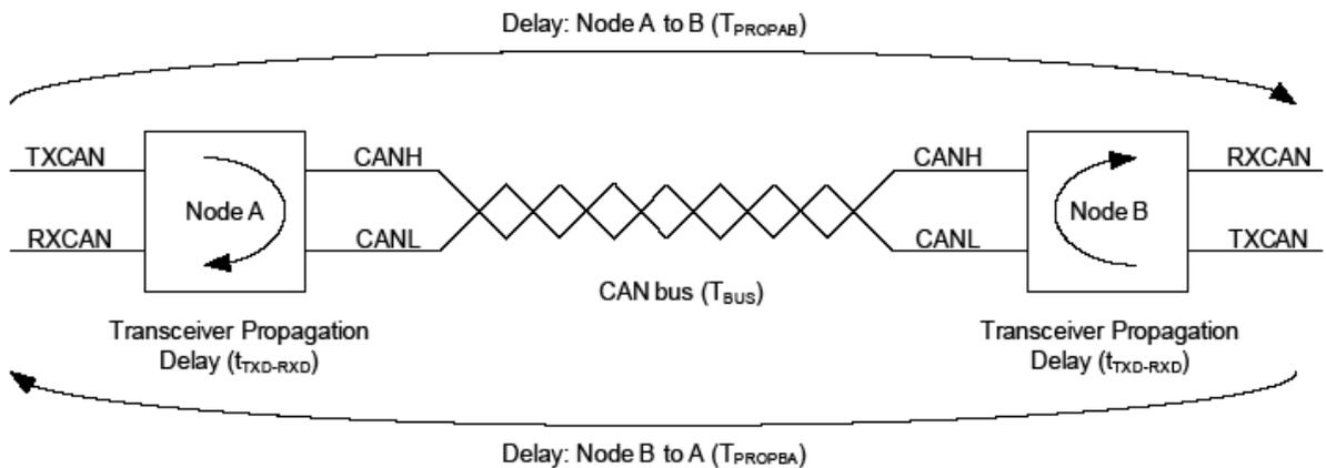
38.3.3.3 Transmitter Delay Compensation (TDC)
