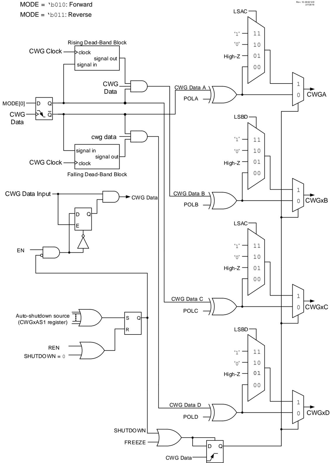
In Forward Full-Bridge mode ( $MODE = \text{'b010}$ ), CWGxA is driven to its Active state, CWGxB and CWGxC are driven to their Inactive state, and CWGxD is modulated by the input signal, as shown in Figure 32-7.
