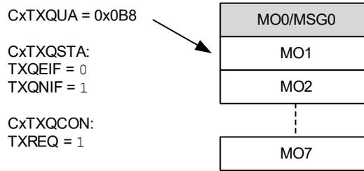
Figure 38-34 illustrates the status of the TXQ after MSG0 is transmitted. The TXQ is empty again. TXQEIF is set and TXREQ is cleared. The user address still points to MO1 because UINC is not set.
