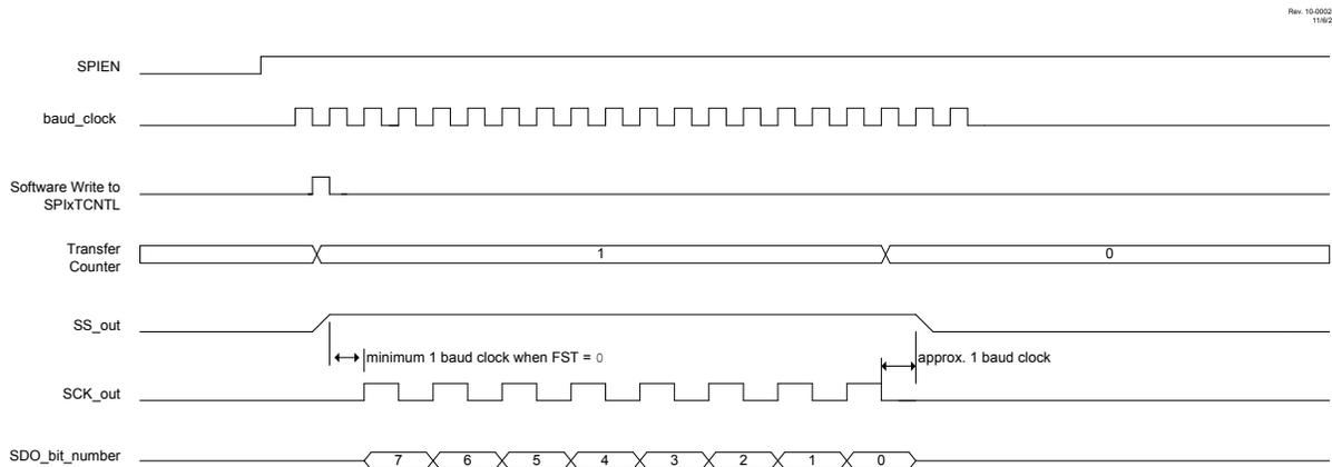
Note: 1. *SDO bit number* illustrates the transmitted bit number, and is not intended to imply SDO\_out tristate operation.
