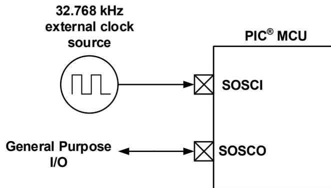
The SOSC can be enabled through one of two methods:
