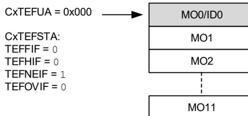
Figure 38-40 illustrates the status of the TEF after ID0 is read. The user application reads the ID from RAM and sets the UINC bit (C1TEFCONL[8]). The user address increments and points to MO1. The TEF is empty again. All flags are cleared.
