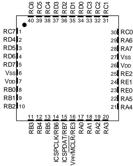
**Note:** It is recommended that the exposed bottom pad be connected to  $V_{SS}$ ; however, it must not be the only  $V_{SS}$  connection to the device.
