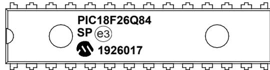
28-Lead SOIC (7.50 mm)
