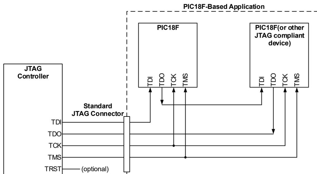
In PIC18-Q84 devices, hardware for the JTAG boundary scan is a Core Independent Peripheral (CIP) with additional integrated logic in all I/O ports. A logical block diagram of the JTAG module is shown in Figure 39-2. It consists of the following key elements:
