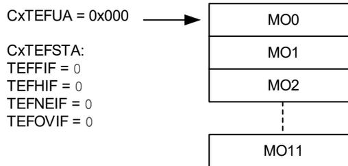
Figure 38-39 shows the status of the TEF after the first transmit message is stored. MO0 contains ID0, the ID of MSG0. TEFNEIF is set since the TEF is not empty. The user address points to MO0.
