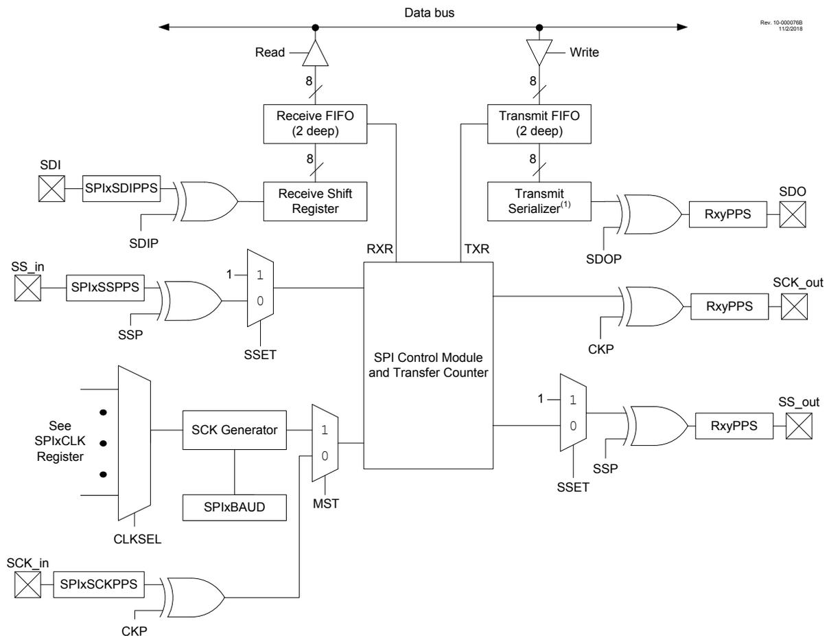
Note 1: If the transmit FIFO is empty and TXR = 1, the previous value of the receive shift register will be sent to the transmit serializer.
