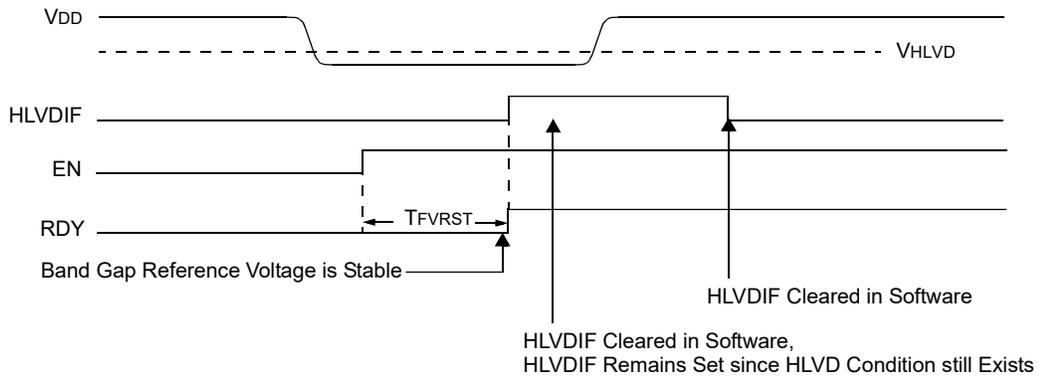
Figure 40-3. High-Voltage Detect Operation (INTH = 1)
