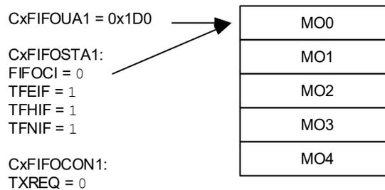
Figure 38-19 illustrates the status of FIFO 1 after the first message (MSG0) is loaded. MO0 now contains MSG0. The user application sets the UINC bit (CxFIFOCON1[8]), which causes the FIFO head to advance. The user address now points to MO1. TFEIF is cleared since the FIFO is no longer empty. The user application now sets TXREQ to request the transmission of MSG0.
