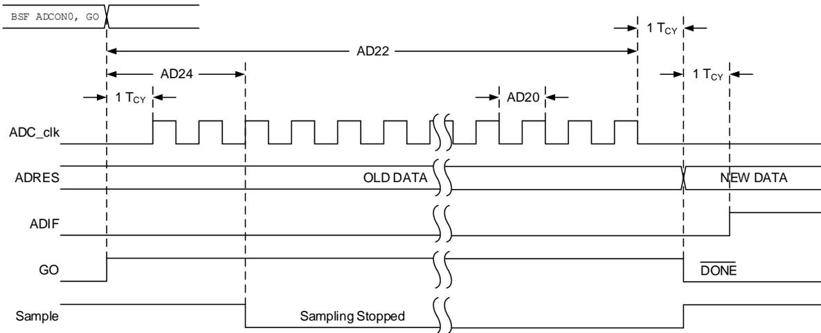
Figure 50-10. ADC Conversion Timing (ADC Clock from ADCRC)
