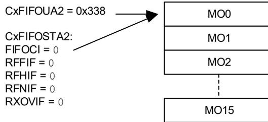
Figure 38-25 illustrates the status of FIFO 2 after the first message (MSG0) is received. MO0 now contains MSG0. The FIFO index now points to MO1. RFNIF is set since the FIFO is not empty anymore.
