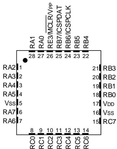
**Note:** It is recommended that the exposed bottom pad be connected to V<sub>SS</sub>; however, it must not be the only V<sub>SS</sub> connection to the device.
