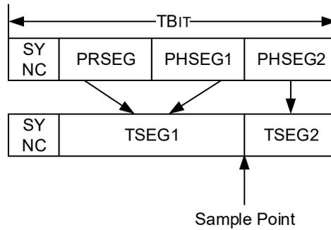
The total number of TQ in a bit time is programmable and can be calculated using [Equation 38-5](#) and [Equation 38-6](#).
