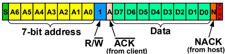
Figure 37-24. 7-Bit Host Read Diagram (from a specific memory/register location)
