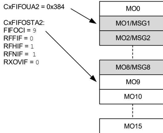
Figure 38-28 illustrates the status of FIFO 2 after ten more messages are received: MSG5-MSG15. The user address still points to MO1. The FIFO index points to MO0. RFNIF and RFHIF are set.
