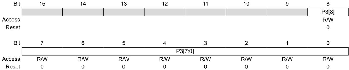
**Bit 8 – P3[8]** Parameter 3 Most Significant bit
