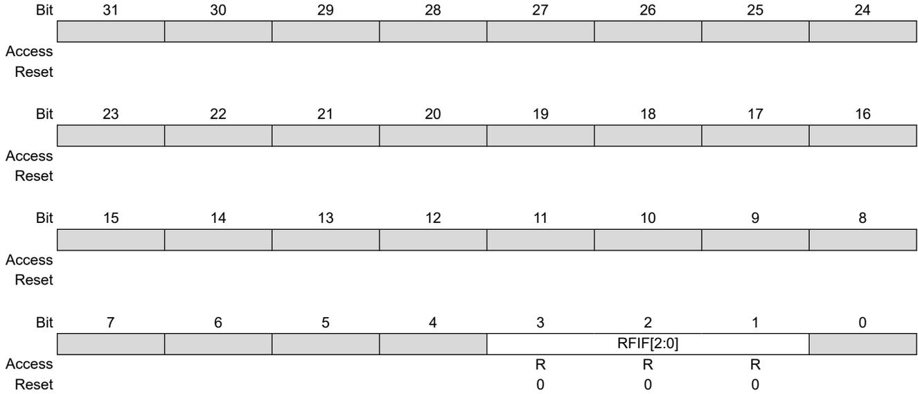
**Bits 3:1 – RFIF[2:0]** Receive FIFO Interrupt Pending
