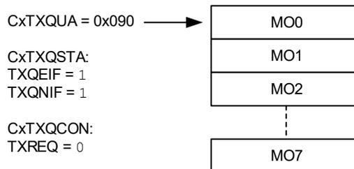
Figure 38-33 illustrates the status of the TXQ after the first message (MSG0) is loaded. MO0 now contains MSG0. The user application sets the UINC bit, which causes the FIFO head to advance. The user address now points to MO1. TXQEIF is cleared, since the queue is not empty anymore. The user application now sets TXREQ to request the transmission of MSG0.
