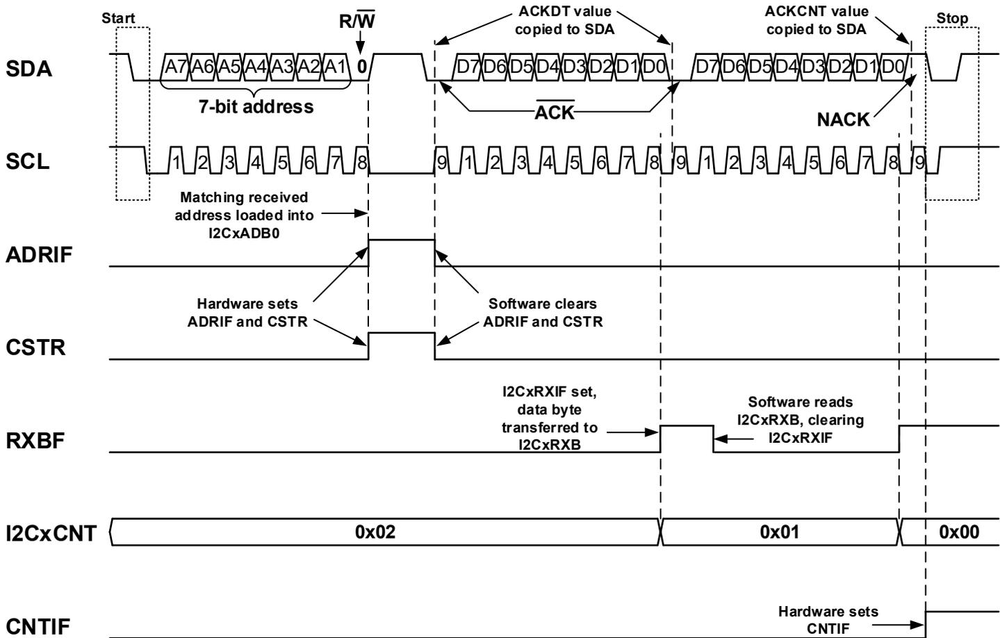
Figure 37-18. 7-Bit Client Mode Reception (ACKTIE = 1)
