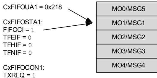
Figure 38-23 illustrates the status of FIFO 1 after MSG1-MSG5 are transmitted. The FIFO is empty again. All status flags are set and TXREQ is cleared. The user address and the FIFO index point to MO1 again.
