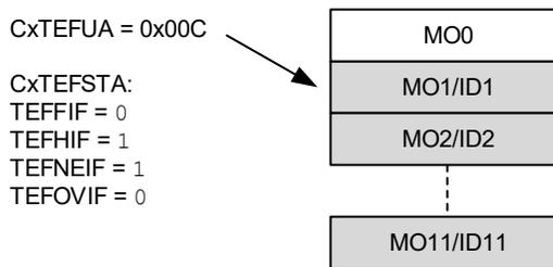
Figure 38-43 illustrates the status of the TEF after one more message is transmitted: MSG12. All status flags are set because the TEF is full. The user address points to MO1.
