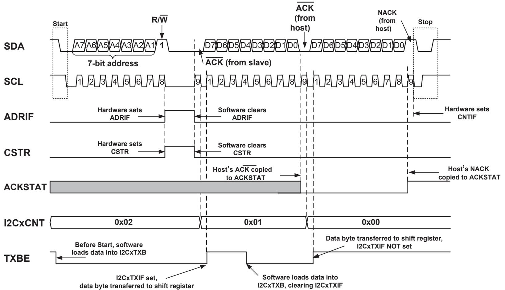
Figure 37-15. 7-Bit Client Mode Transmission (ACKTIE = 1)
