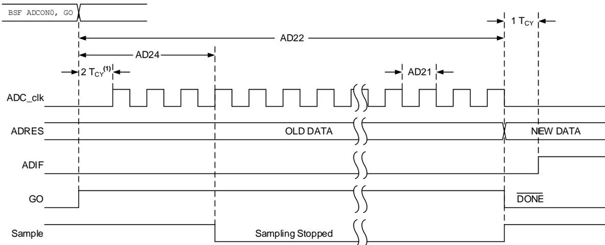
**Note 1:** If the ADC clock source is selected as ADCRC, a time of  $1 T_{cy}$  is added before the ADC clock starts. This allows the **SLEEP** instruction to be executed, if any.
