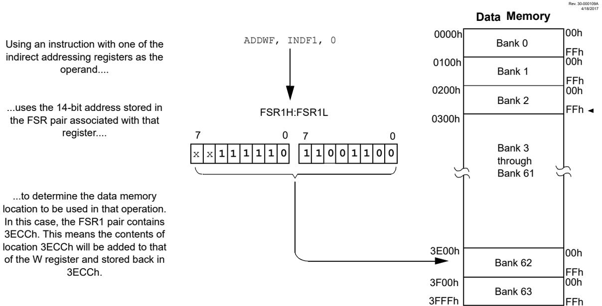
Operations on the FSRs with `POSTDEC`, `POSTINC` and `PREINC` affect the entire register pair; that is, rollovers of the `FSRnL` register from `FFh` to `00h` carry over to the `FSRnH` register. On the other hand, results of these operations do not change the value of any flags in the `STATUS` register (e.g., `Z`, `N`, `OV`, etc.).
