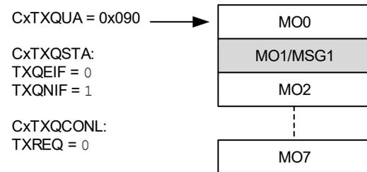
Figure 38-36 illustrates the status of the TXQ after six more messages are loaded: MSG2-MSG7. The user address now points to the last free message object: MO7.
