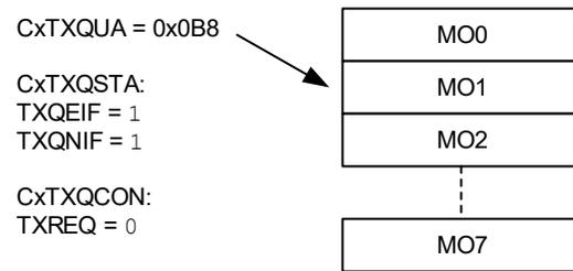
Figure 38-35 illustrates the status of the TXQ after MSG1 is loaded and UINC is set. The user address now points to the next free message object: MO0.
