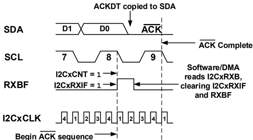
Figure 37-34. Not Acknowledge (NACK) Sequence Timing
