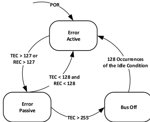
The error-free message counter, together with the error counters and error flags, can be used to determine the quality of the bus.
