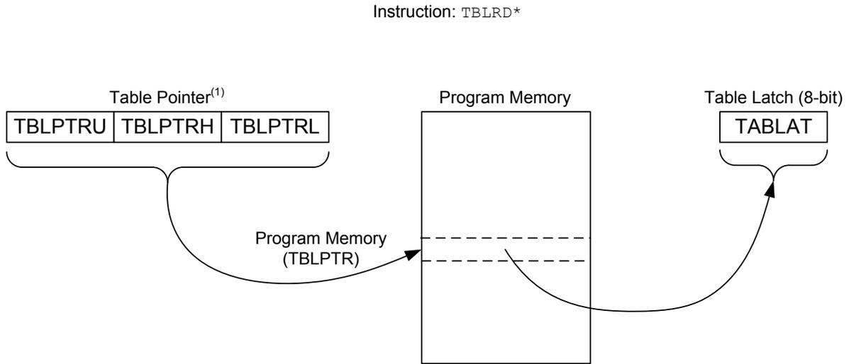
Note 1: The Table Pointer register points to a byte in program memory.
