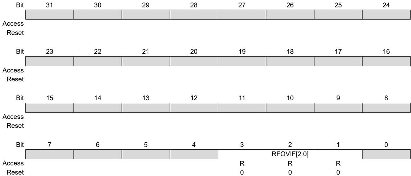
**Bits 3:1 – RFOVIF[2:0]** Receive FIFO Overflow Interrupt Pending
