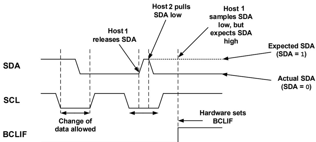
Figure 37-43. Multi-Host Mode Transmission
