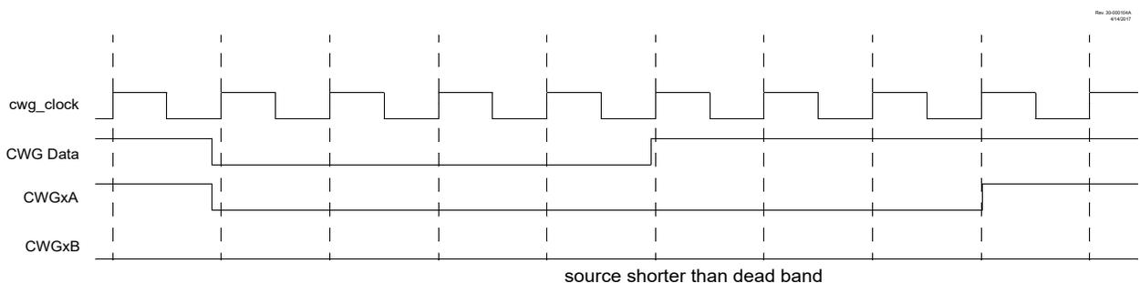
The CWGxDBF register value is double-buffered. When EN = 0, the buffer is loaded when CWGxDBF is written. When EN = 1, then the buffer will be loaded at the rising edge following the first falling edge of the data input after the LD is set.
