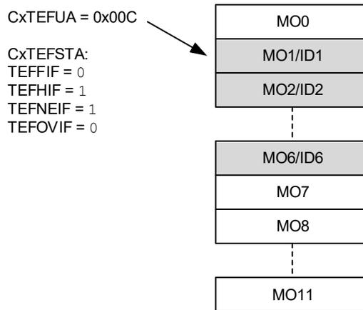
Figure 38-42 illustrates the status of the TEF after five more messages are transmitted: MSG7-MSG11. The user address still points to MO1. TEFNEIF and TEFHIF are set.
