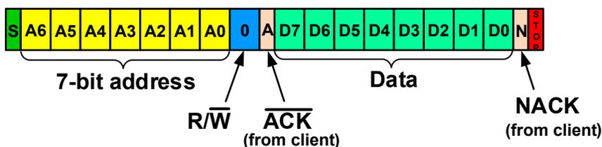
Figure 37-27. 7-Bit Host Write Diagram (to a specific memory/register location)
