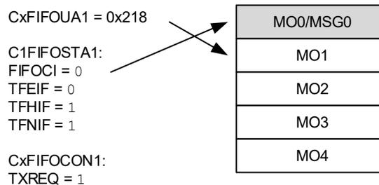
Figure 38-20 illustrates the status of FIFO 1 after MSG0 is transmitted. The FIFO is empty again. TFEIF is set and TXREQ is cleared. FIFOCIx bits now point to MO1 with user address 0x218.
