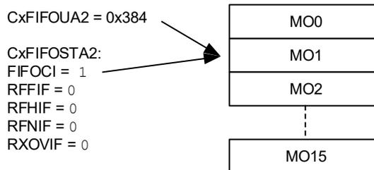
Figure 38-27 illustrates the status of FIFO 2 after eight more messages are received: MSG1-MSG8. The user address still points to MO1. RFNIF and RFHIF are set because the FIFO is now half full. The FIFO index points to MO9.
