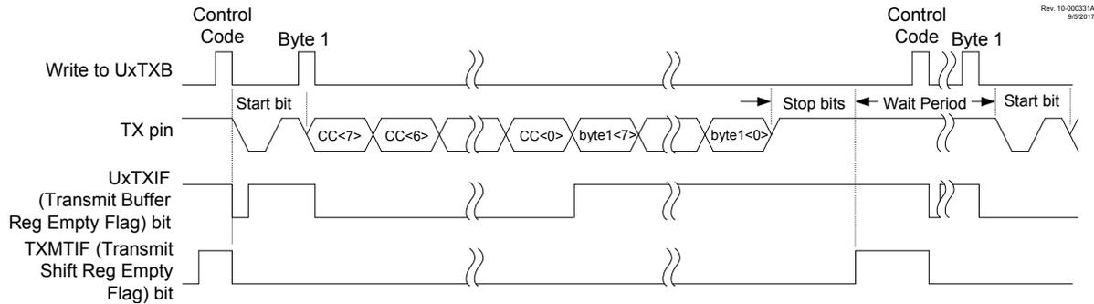
During the communication between two Control Devices, three bytes are required to be transmitted. In this case, the software must write the third byte to UxTXB as soon as UxTXIF goes true and before the output shifter becomes empty. This ensures that the three bytes of the forward frame are transmitted back-to-back without any interruption.
