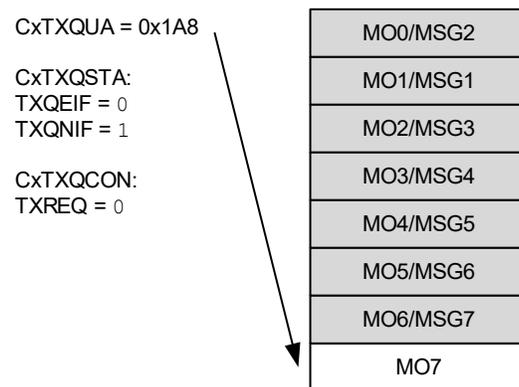
Figure 38-37 illustrates the status of the TXQ after MSG8 is loaded and UINC is set. The TXQ is now full, all flags are cleared. The user address now points to MO0. The user application now sets TXREQ. The messages will be transmitted based on the priority of their IDs.
