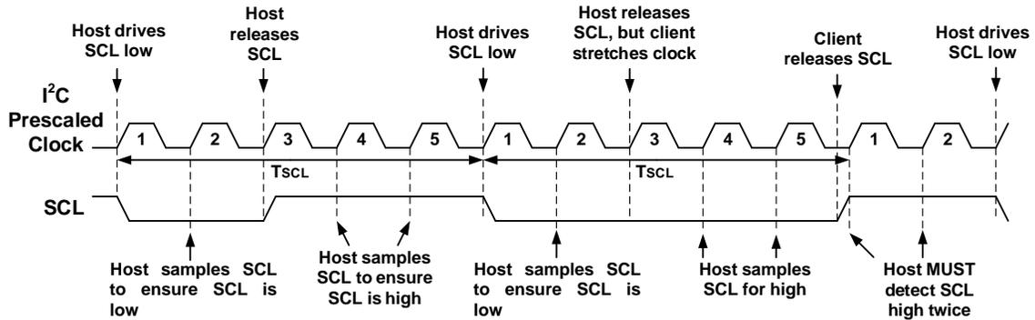
When **FME** is set ( $FME = 1$ ), one SCL period ( $T_{SCL}$ ) is equal to four clock periods of the prescaled **I2CxCLK** source. In other words, the prescaled **I2CxCLK** source is divided by four. Using the example from above, if the **HFINTOSC** (4 MHz) clock source is selected, **I2CxBAUD** is loaded with a value of '7' and the **FME** bit is set, the actual SCL frequency is 125 kHz (see the Equation below).
