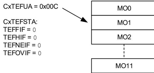
Figure 38-41 illustrates the status of the TEF after six more messages are transmitted: MSG1-MSG6. The user address points to MO1. TEFNEIF and TEFHIF are set because the TEF is now half full.
