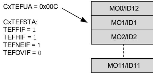
Figure 38-44 illustrates the status of the TEF after one more message is transmitted. Since the TEF is already full, an overflow occurs. The ID is discarded and TEFOVIF is set. The user address remains unchanged.
