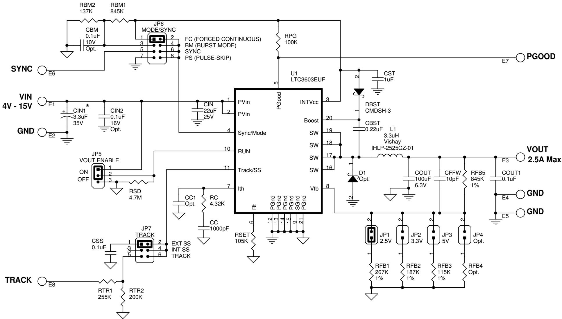
\* Capacitor CIN1 Is An Optional Capacitor. It Is Inserted On The DC1442A To Dampen The (Possible) Ringing Voltage Due To The Long Input Leads. On A Normal, Typical PCB, With Short Trace, The Capacitor Is Not Needed.
