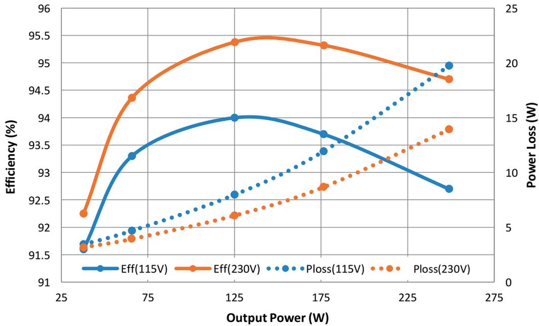
Figure 10. Efficiency for the power supply at 115V and 230V input
