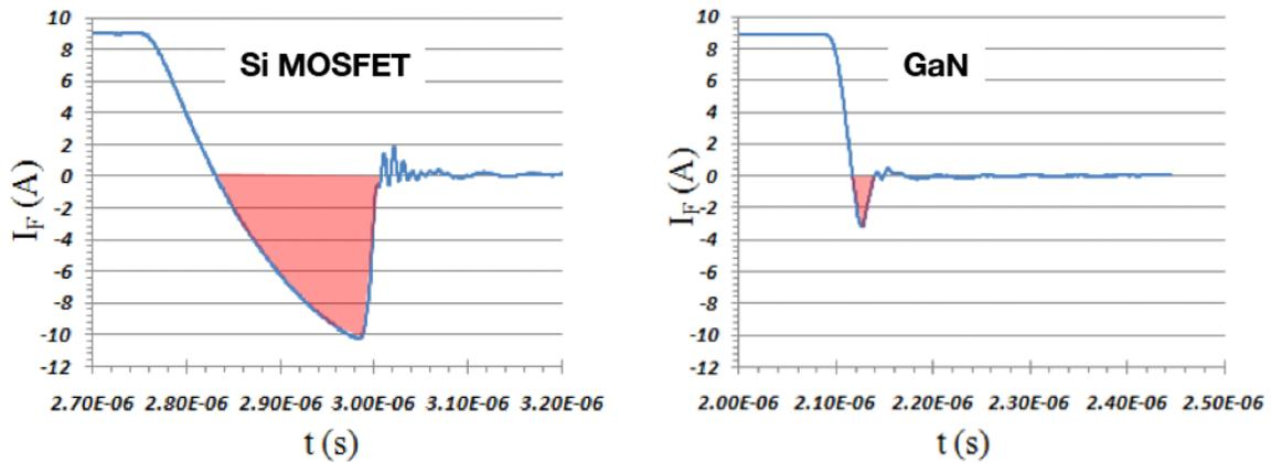
**Figure 6. Reverse recovery charge test result for a Si MOSFET and a GaN FET:
