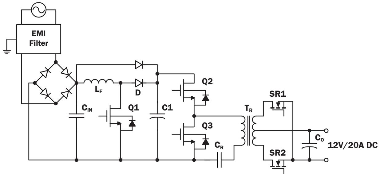
**Figure 2. Simplified schematic for the complete power supply**
