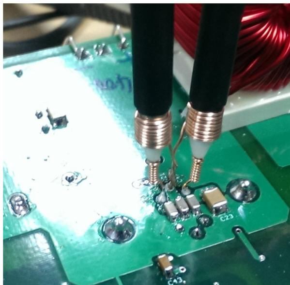
**Figure 7. Low inductance probing of fast, high-voltage signals**
