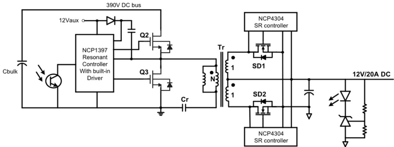
**Figure 5. Circuit topology for LLC DC-DC converter using Si MOSFETs for line rectification**
