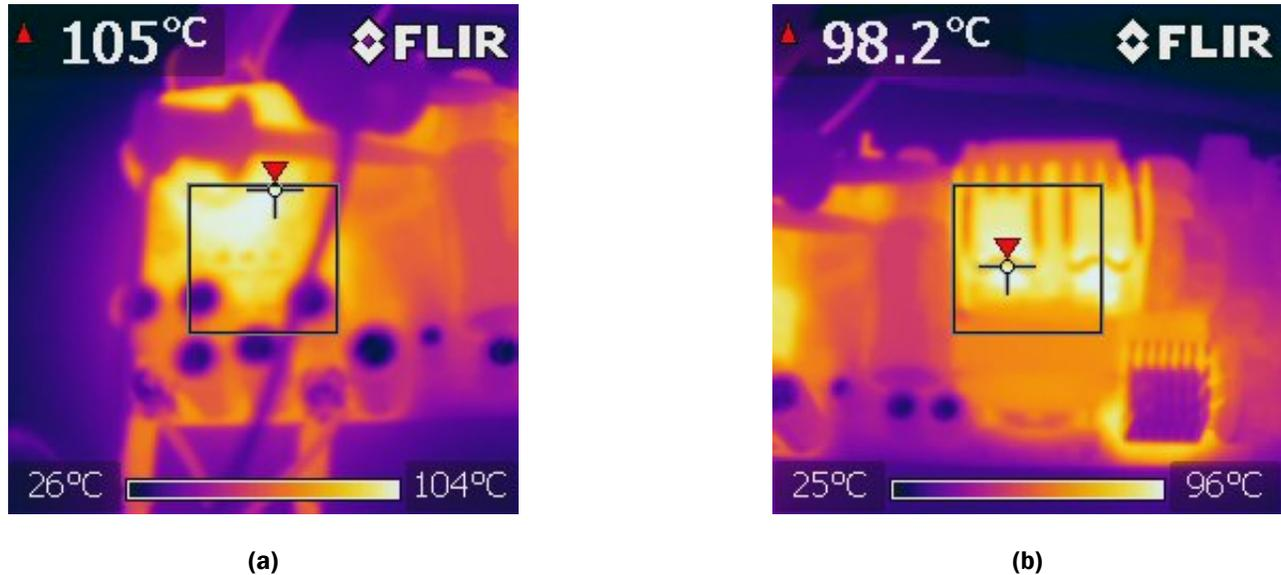
**Figure 14. Temperature measurement at full load, 115V input  $T_A=23\text{ }^\circ\text{C}$**
