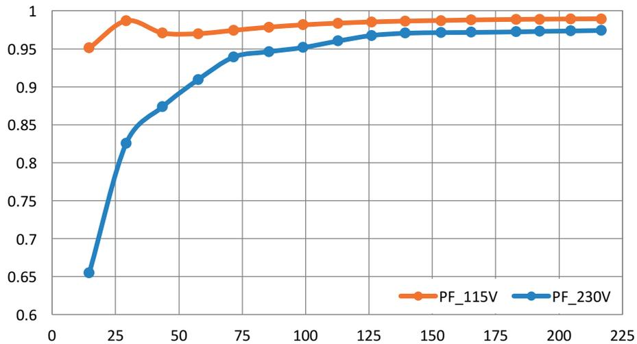
Figure 11. Power factor vs. output power at 115V and 230V input
