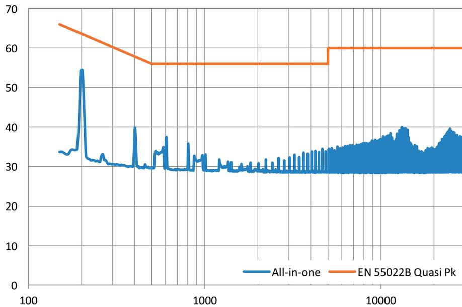
**Figure 13. Conducted emissions at 115V<sub>AC</sub> and 240W load**
