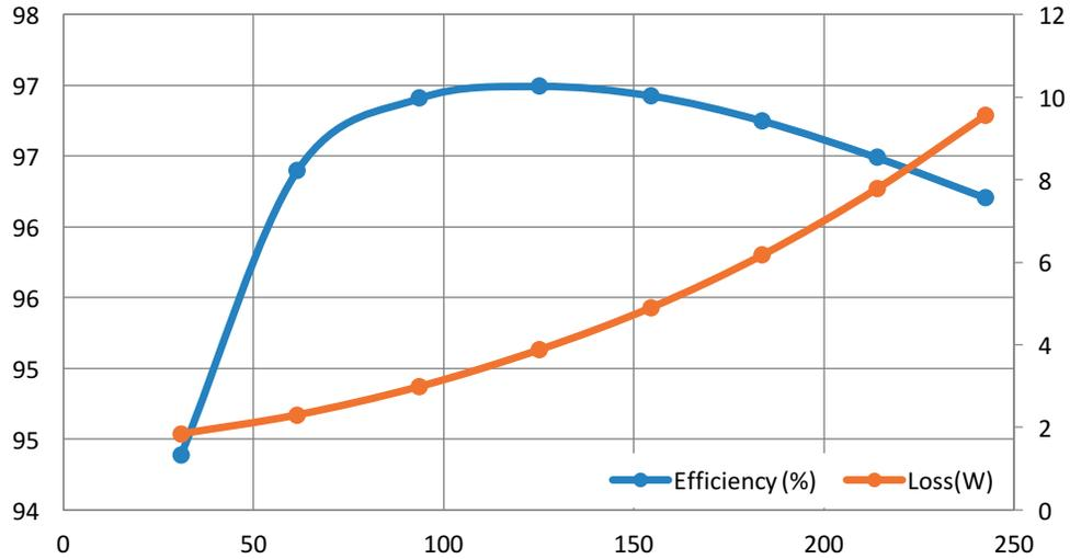
**Figure 12. Efficiency results for the LLC DC-DC converter circuit at 390V<sub>DC</sub> input to 12V<sub>DC</sub> output**
