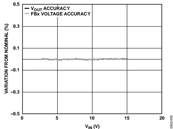
Figure 7. Boost Regulator Line Regulation,  $V_{\text{POS}} = 15\text{ V}$ ,  $f_{\text{SW}} = 1.2\text{ MHz}$ ,  $15\text{ mA Load}$ ,  $T_A = 25^\circ\text{C}$  (Nominal Defined as Average Value Within a Range of 10% to 90%  $V_{\text{IN}}$ )
