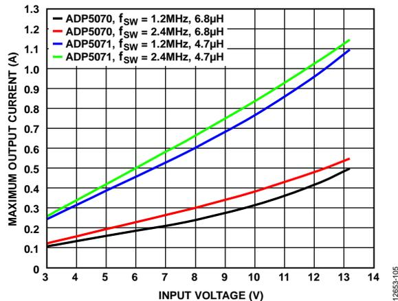
Figure 5. Boost Regulator Maximum Output Current (A) vs. Input Voltage (V)
