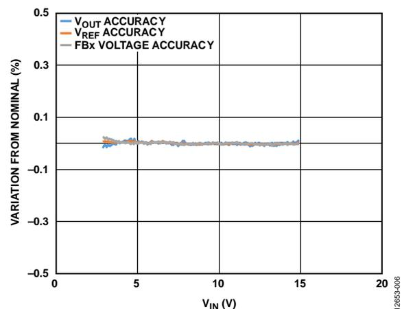
Figure 8. Inverting Regulator Line Regulation,  $V_{\text{NEG}} = -15\text{ V}$ ,  $f_{\text{SW}} = 1.2\text{ MHz}$ ,  $15\text{ mA Load}$ ,  $T_A = 25^\circ\text{C}$  (Nominal Defined as Average Value Within a Range of 10% to 90%  $V_{\text{IN}}$ )
