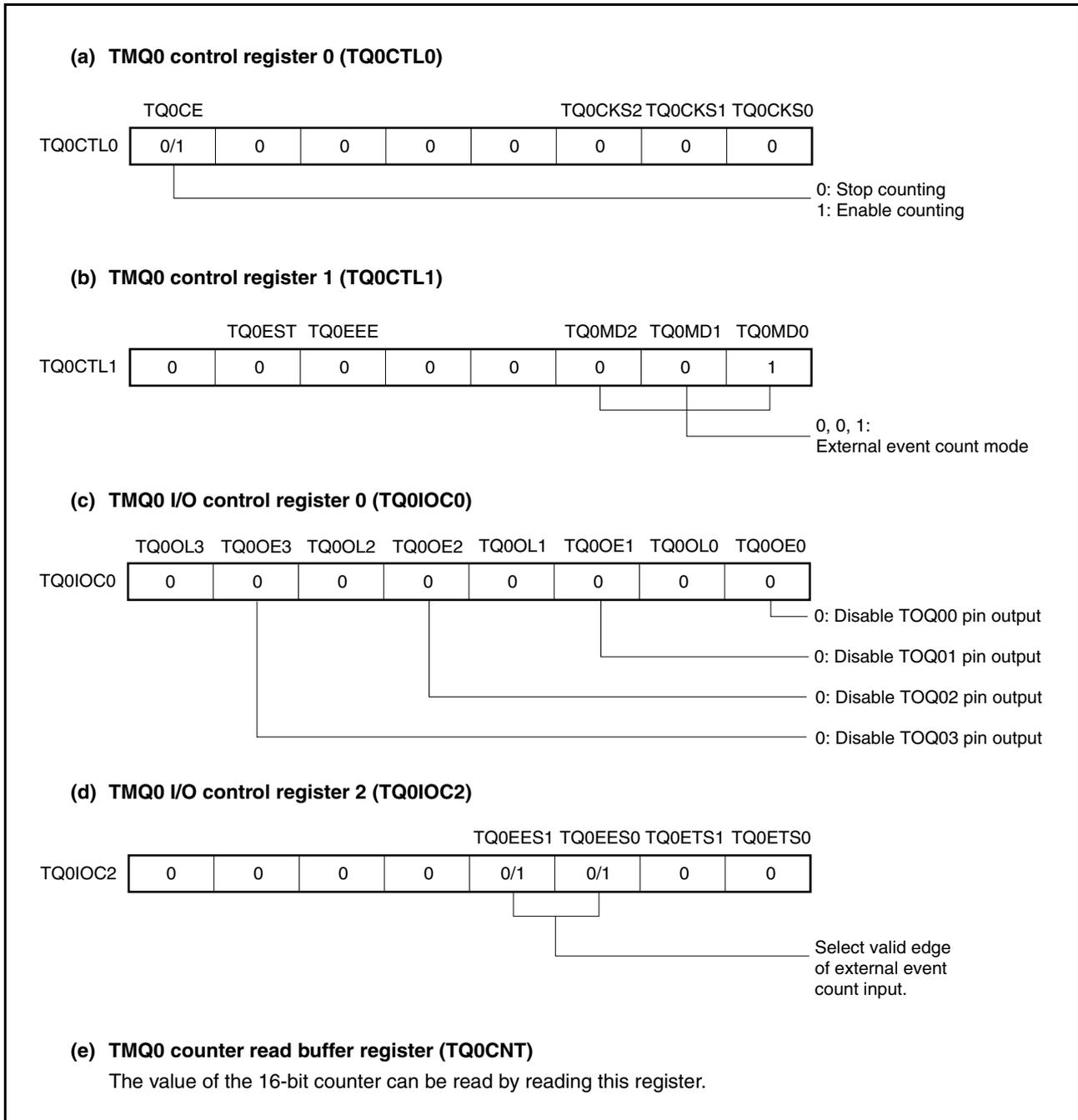
Figure 7-19. Register Settings in External Event Count Mode (2/2)
