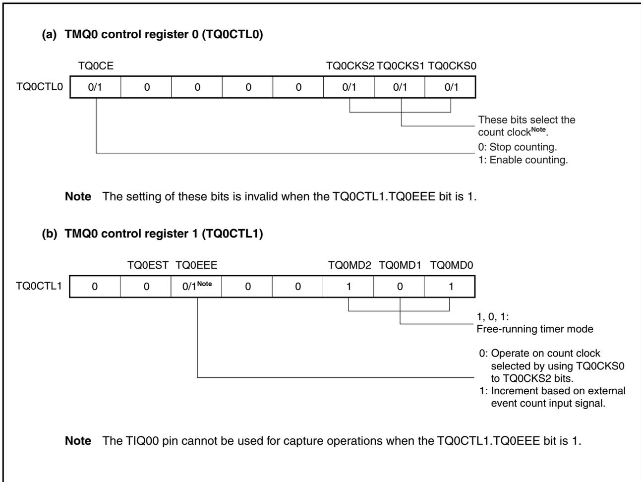
Figure 7-55. Register Settings in Free-Running Timer Mode (2/3)
