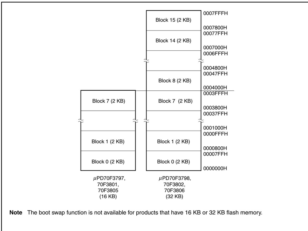
Figure 28-1. Flash Memory Mapping (2/2)
