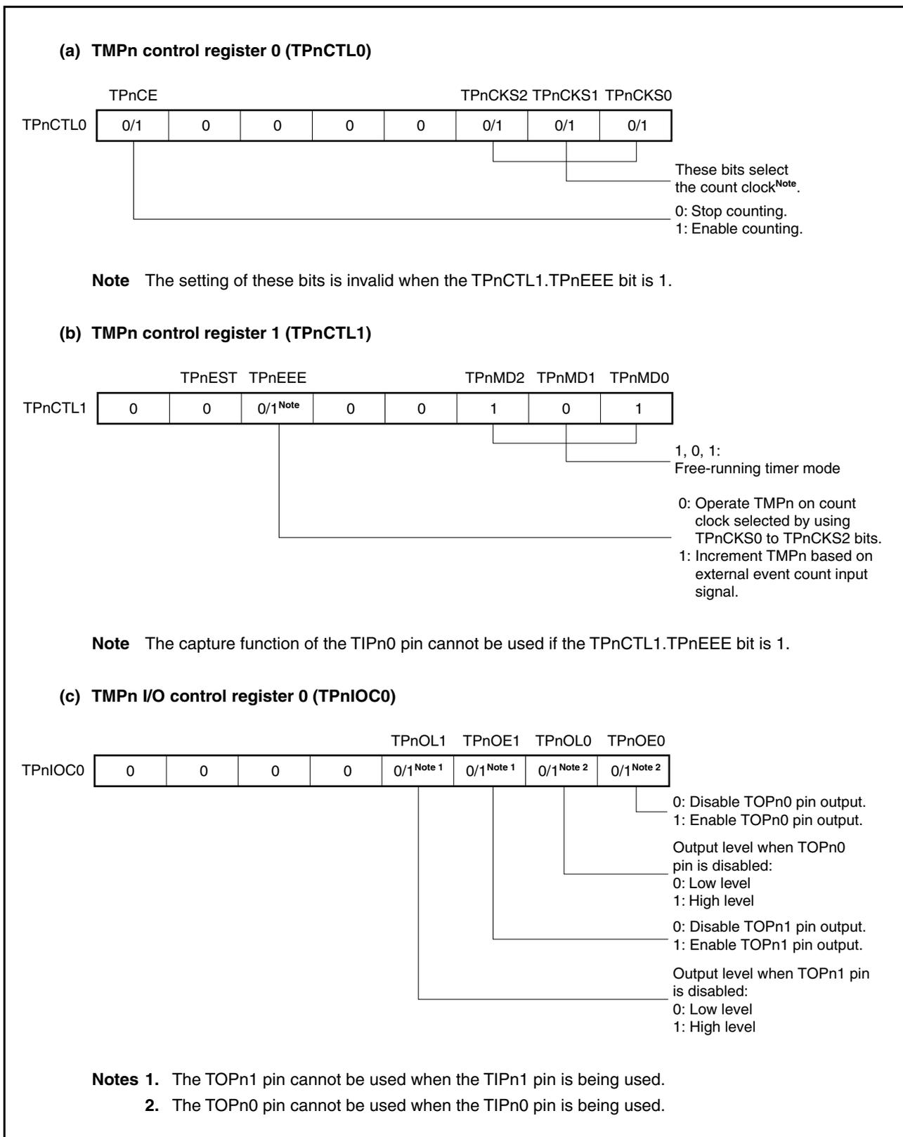
Figure 6-55. Register Settings in Free-Running Timer Mode (2/2)
