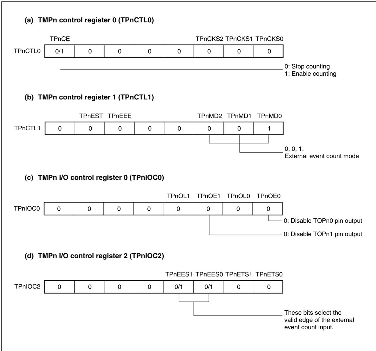
Figure 6-19. Register Settings in External Event Count Mode (2/2)
