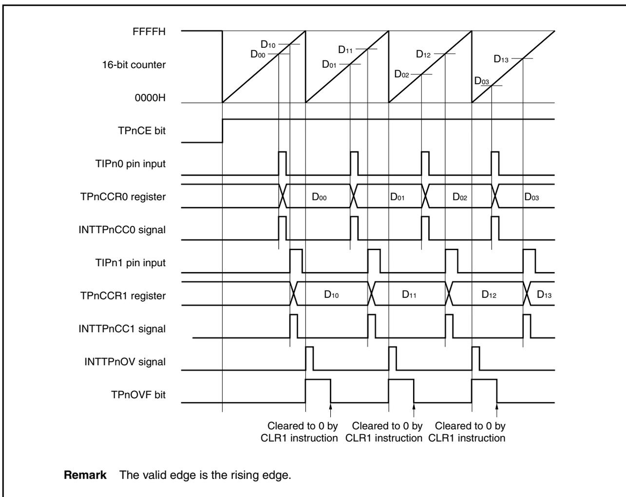
Figure 6-55. Register Settings in Free-Running Timer Mode (1/2)
