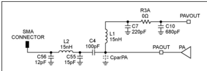
Figure 7. Diagram of the MAX7060 match and filter for +14dBm with ETSI compliance.
