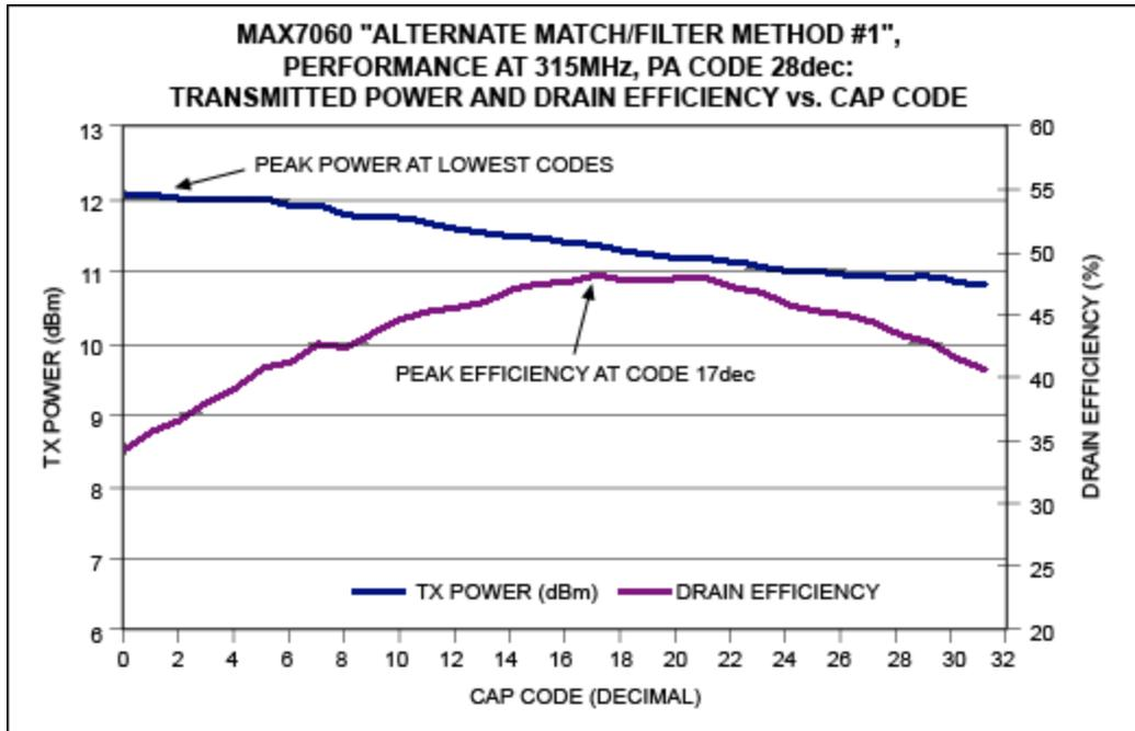
Figure 10. TX power and drain efficiency vs. cap code at 315MHz, using Alternate Match/Filter Method #1.
