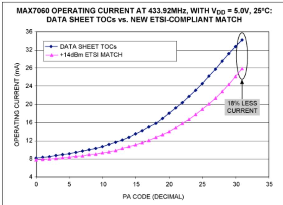
Figure 9. Decreased operating current with match/filter for +14dBm with ETSI compliance.
