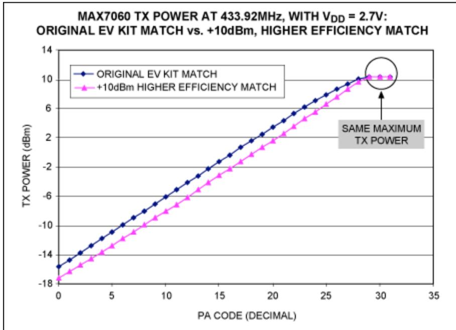
Figure 4. TX power comparison, original match vs. new match/filter for +10dBm.
