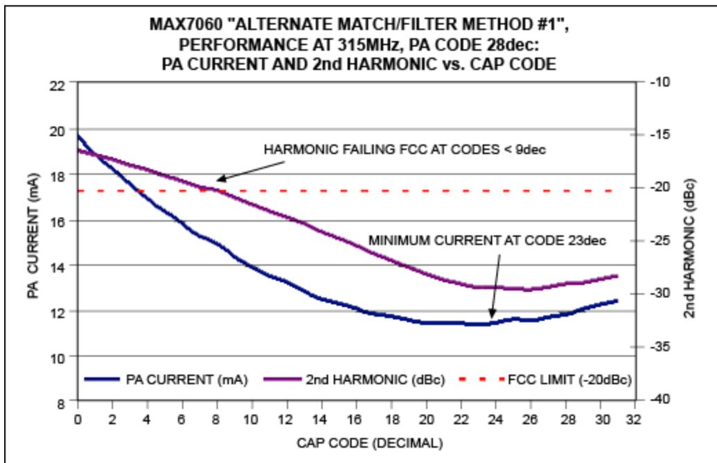
Figure 11. PA current and 2nd harmonic vs. cap code at 315MHz, using Alternate Match/Filter Method #1.
