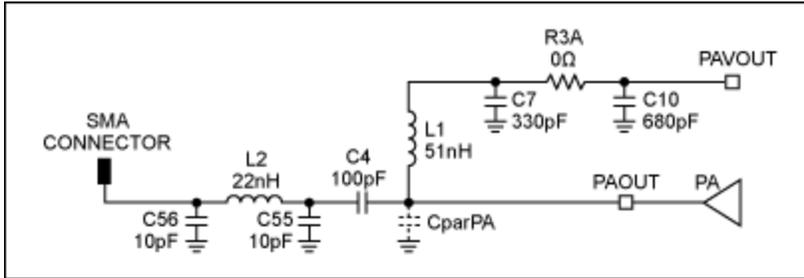
Figure 1. Simplified diagram of the MAX7060EVKIT match and filter networks.
