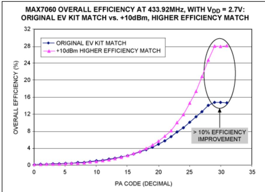
Figure 6. Improved overall efficiency with new match/filter for +10dBm.
