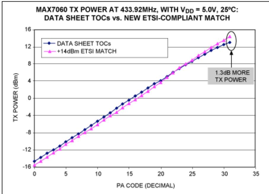
Figure 8. Improved power with match/filter for +14dBm with ETSI compliance.
