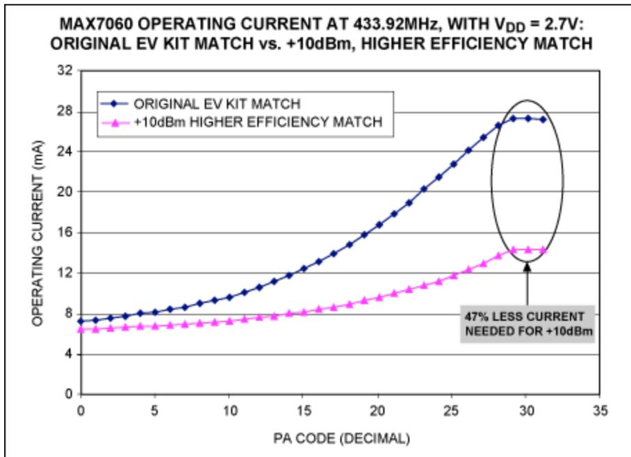
Figure 5. Decreased operating current with new match/filter for +10dBm.
