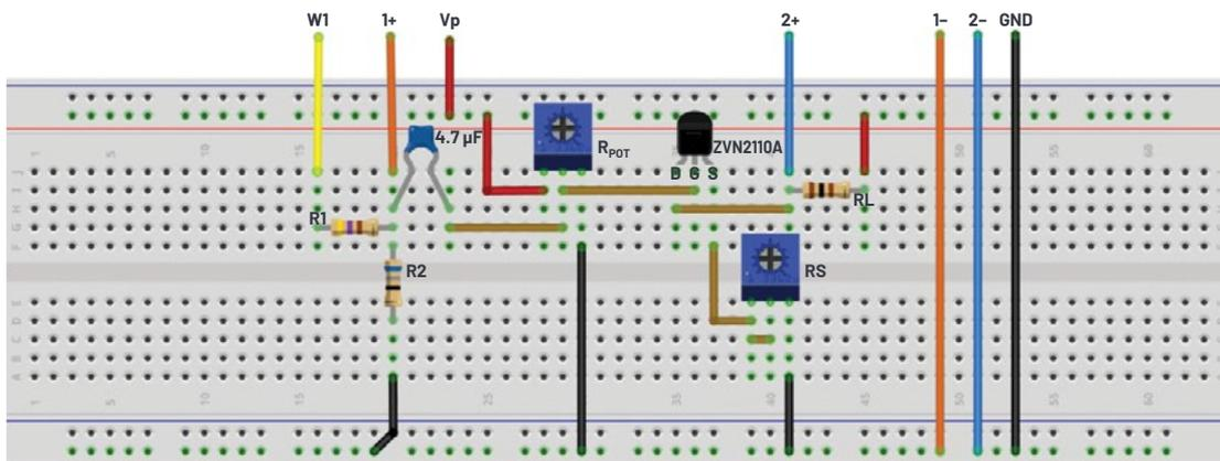
Figure 5. Source degeneration added to a breadboard connection.
