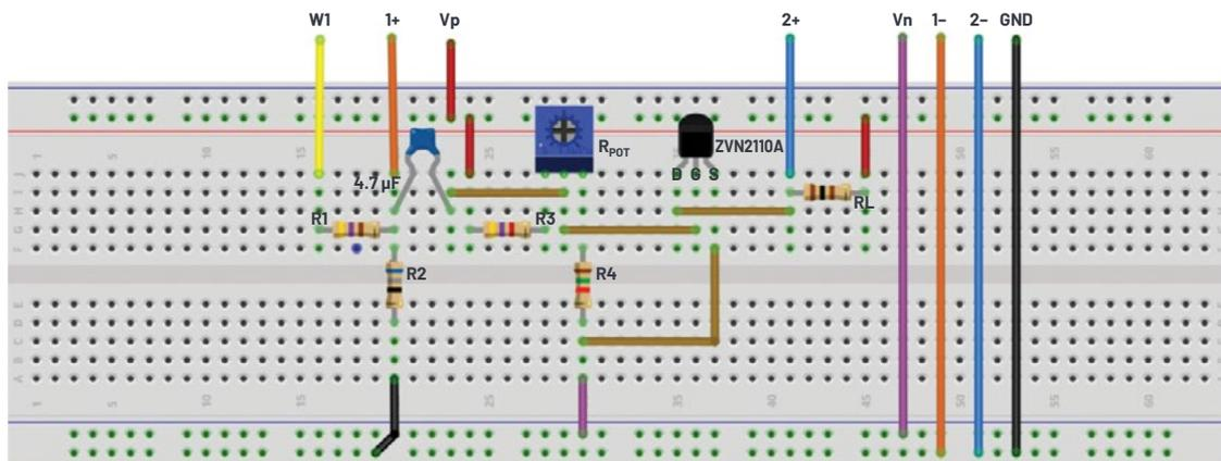
Figure 2. NMOS diode breadboard circuit.
