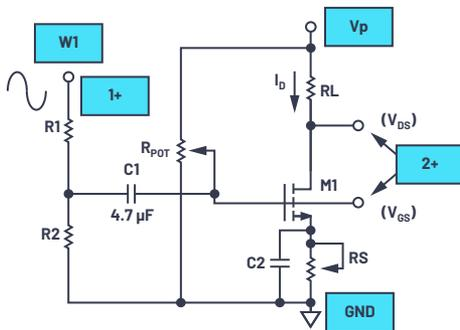
Figure 7.  $C_2$  added to increase ac gain.
