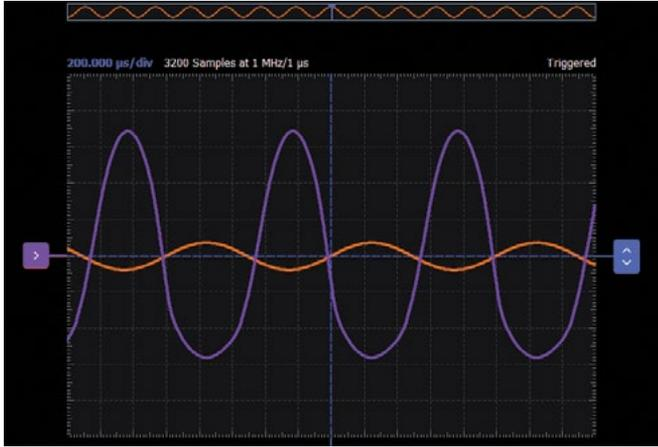
Figure 3. Scopy plot of a common source amplifier test circuit.
